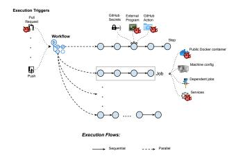
Figure 1: GitHub workflow architecture. When workflow is triggered by execution triggers, it will start the execution of one or more jobs in separate VMs. Each job consists of steps that are executed in the defined order. Steps can be a shell commands, third-party actions, external programs, docker containers
